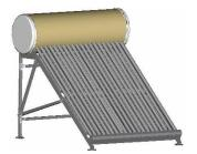
When you insert the glass tubes, please do like this: Put the rubber ring around the glass tube and brush some lubricate (detergent) around it so as to rotate tube into tank slowly. Then aim tube at down holder and place into it. Put the rubber ring up tube till tightly against the tank.
