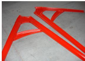
Step 5: Assembling front strength ribs (1 pc)
