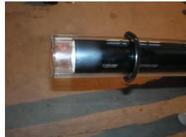
Step 13: Dipping tube orifice with Lube
